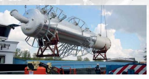
project in the Middle East. And isn't it great that Gouda Refractories was chosen to supply the refractory material? And how about the distillation column that was supplied, measuring 29 metres in length, weighing 72 tonnes and boasting a diameter of 8.5 m? Seeing such a colossal construction leaving the site by ship inevitable leads to everyone being awestruck by the accomplishment, and rightly so!
